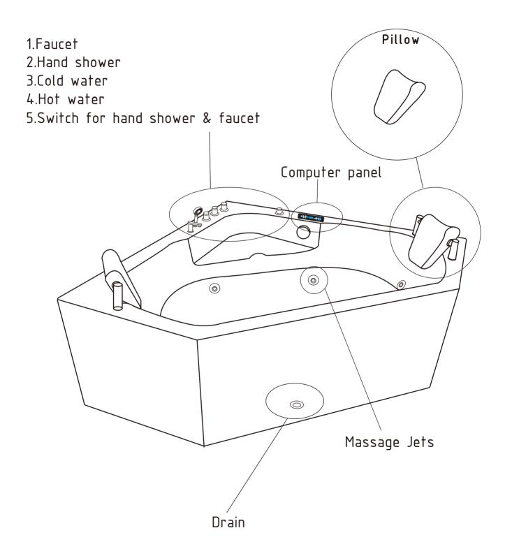
Water & Electricity Position Design Length unit: mm
