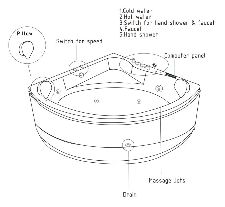
Water & Electricity Position Design Length unit: mm
