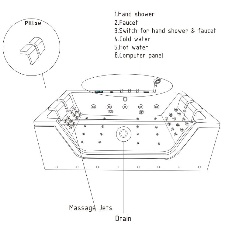
Water & Electricity Position Design Length unit:mm
